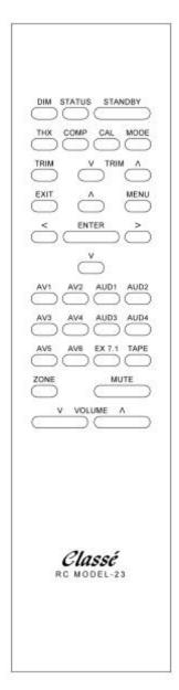
**AV1 - AV6** These six keys each directly access one of the AV Sources consisting of a Video Input and a hard-wired Analog Audio input plus any associated Digital Audio input selected during setup. These keys can also be used to select Zone Sources.
